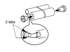
**4** Hold the empty spool so that the end with only one slot is on the left, and lower the spools into the front of the printing compartment. The gears in the ends of the spool with film should fit into the slots on each side of the printing compartment.
